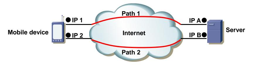
Both mobile device and server have 2 interfaces to the network with 2 IP addresses each. On both the server and mobile device the SCTP socket is bound to both local IP addresses. If one path fails communication is still possible through the other path since SCTP can send/receive from both addresses. SCTP monitors each path and switches to an alternate path if necessary (all peer transport addresses are monitored constantly).
