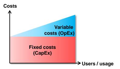
Data centers, servers etc. require a large up-front investment (CapEx). The infrastructure must be dimensioned to accommodate a certain peak load. Variable costs incur on top of CapEx (run-time licenses for users etc.).
