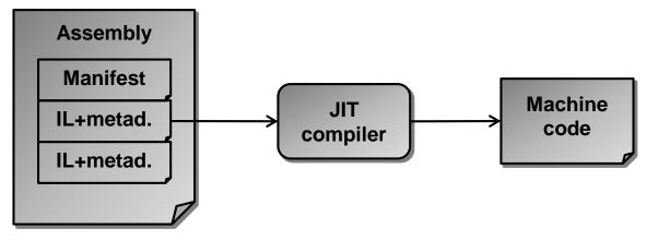
$\rightarrow$  The performance penalty of the translation at runtime applies only for first the call of a method. For subsequent calls, the CLR re-uses the JIT-compiled native method code.
