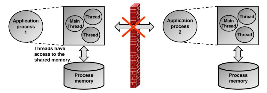
The operating system provides isolation between the processes.
